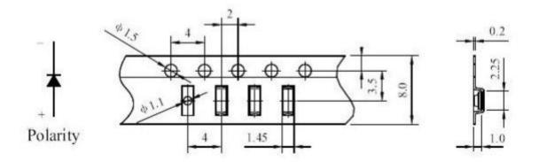
Note:The tolerances unless mentioned is ±0.1mm,Unit:mm
